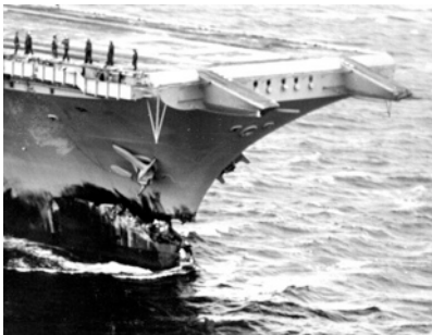
This gaping hole in Ranger's bow from a collision with an oil tanker rendered her inoperative and sent Midway right back to GONZO Station for another long patrol.
